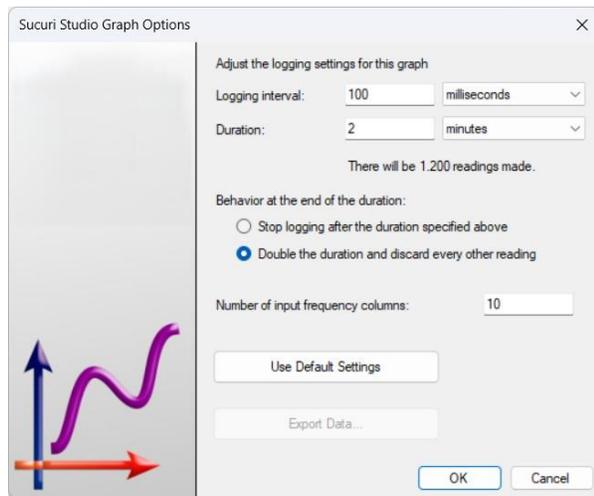
When starting data collection, the readings will be taken every 100ms for 2 minutes, after which the duration and interval are doubled and the other reading will be discarded.
